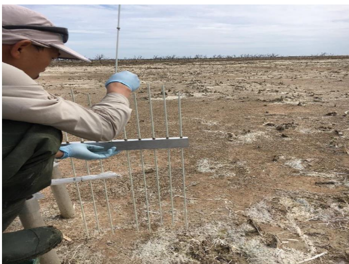
Figure 12. Photo of a Sediment Elevation Table in the trial pond.
